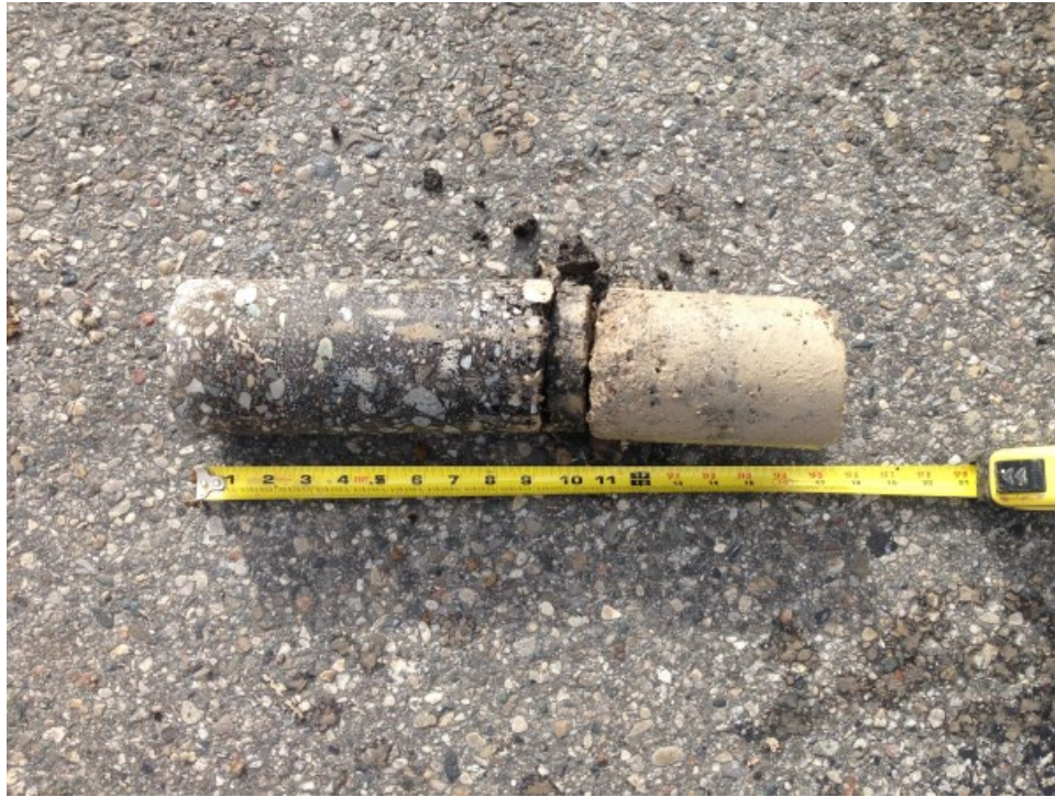
Core Photograph No. 7: 10 inches of Bituminous Concrete 6 inches of Portland Cement Concrete
